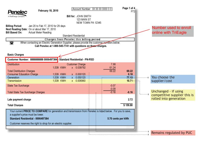
**Distribution Charge** - Charges for the use of local wires, transformers, substations, and other equipment used to deliver electricity to end-use consumers from the high voltage transmission lines.
